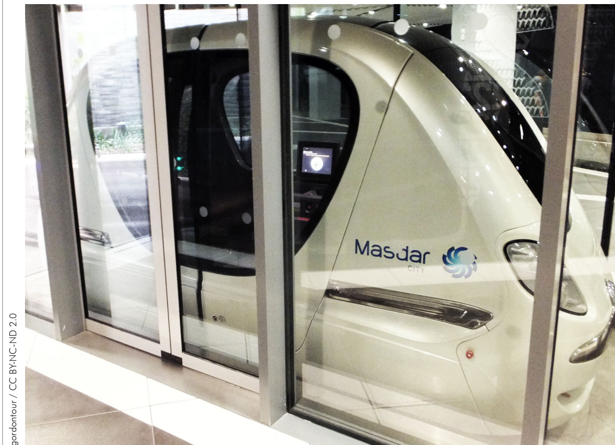
Figure 4.4: Electric PRT vehicles at Masdar City, Abu Dhabi
