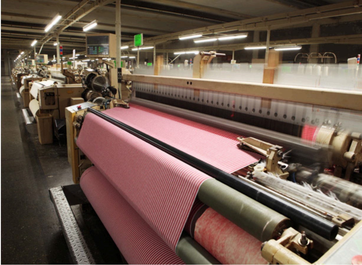
Weaving cotton fabric on an airjet loom — a technology that has far-reaching economic consequences for Member Countries
