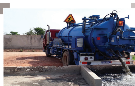
A truck dumping domestic sewage sludge into a waste treatment plant, reducing the pollution of surface water and limiting water-borne diseases
